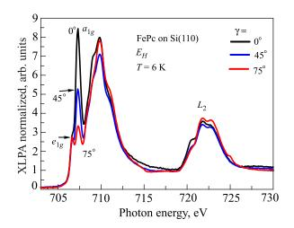
Fig. 3. Normalized XLPA of FePc deposited on Si(110) at the Fe- $L_{2,3}$  edges as a function of incident angle  $0 < \gamma < 75^{\circ}$  measured at T = 6 K.
