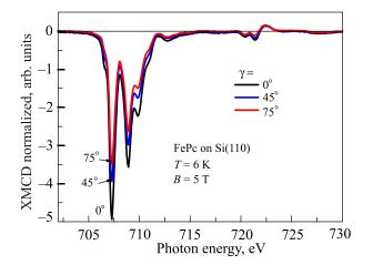
Fig. 4. Normalized XMCD of FePc deposited on Si(110) at the Fe- $L_{2,3}$  edges as a function of incident angle  $0 < \gamma < 75^{\circ}$  measured at T = 6 K.
